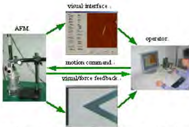
Fig. 1 AFM based robotic nanomanipulation system with real-time force and visual information feedback
