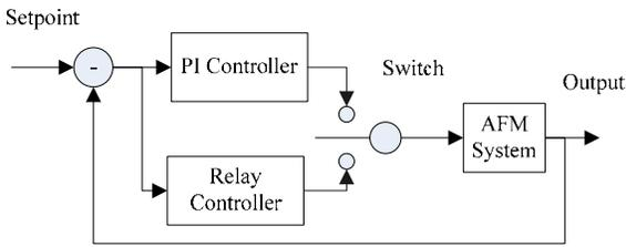
Fig.2 Relay based auto-tuning
