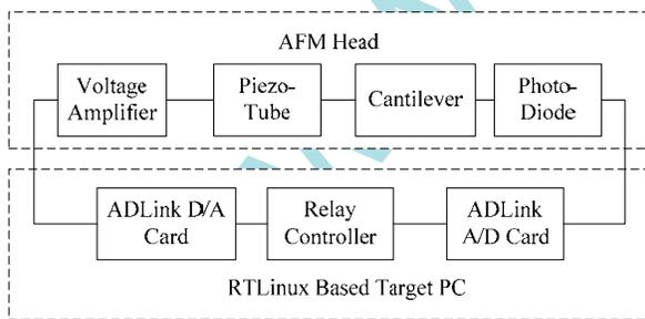
Fig. 3 Relay feedback test system setup.
