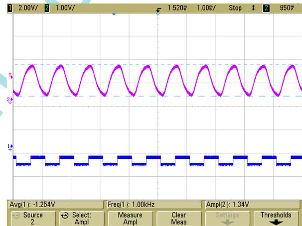
Fig. 4 A typical relay with hysteresis test on AFM system. Relay output is in blue line (lower); deflection output is in purple line (upper).
