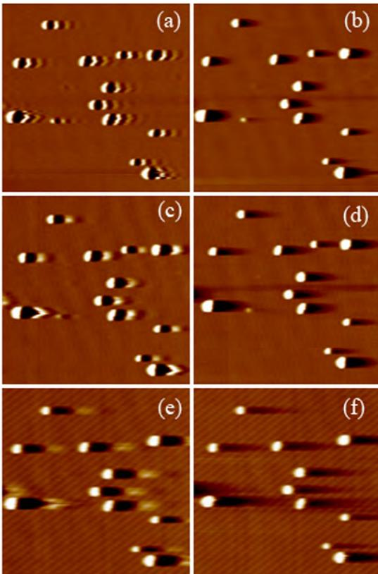
Fig. 8 SiO<sub>2</sub> on mica surface (scan size 450nm). (a) and (b) scanning speed 3Hz ; (c) and (d) scanning speed 5 Hz; (e) and (f) scanning speed 10 Hz. The parameters used for scanning are listed in table 3.
