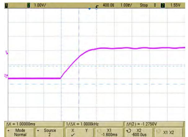
Fig.5 A typical set point step response of the system after auto-tuning.
