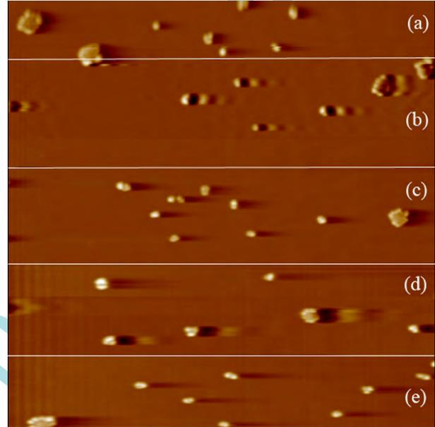
Fig. 7 SiO<sub>2</sub> on mica surface (scan size 10550 nm). (a) scanning speed 3Hz with appropriate PI parameters (b) scanning speed 5 Hz without changing PI parameters (c) scanning speed 5 Hz after tuning parameters (d) 10 Hz without changing PI parameters (e)10 Hz after tuning parameters
