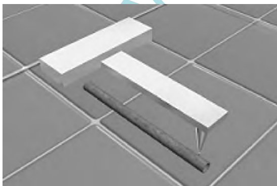
Fig. 2. AFM probe acts on MWCNT.
