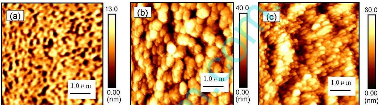
Fig.2. AFM images of the annealed Al films in air for 1h at: (a)600, (b)1200 and (c)1300°C.
