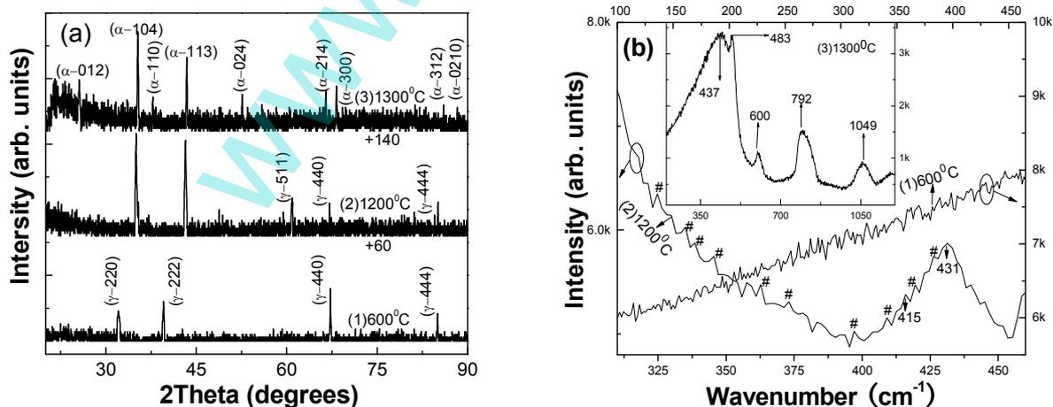
Fig. 1. (a)XRD and (b)RS of the annealed Al films in air for 1h at (1)600,(2)1200 and (3)1300 $^{\circ}\text{C}$ .
