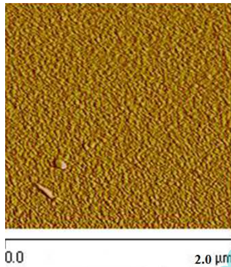
Fig.3. AFM image of \text{TiO}_2 thin film without annealing
