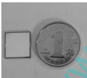
图6 MIM 电容器原型器件 Fig. 6 Prototype device of MIM capacitor
