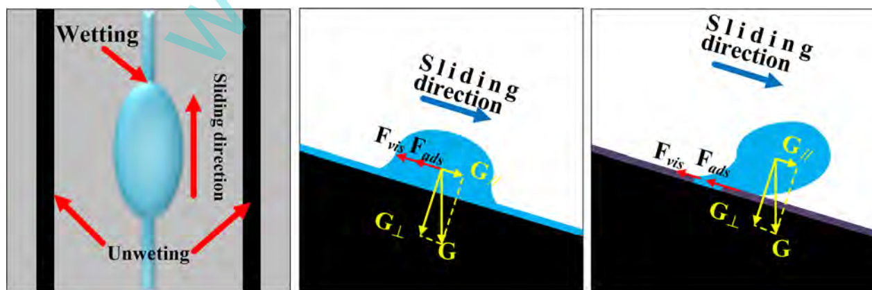
FIG. 10. (Color online) Schematic illustration of a droplet sliding off the line pattern in directions: (a) top view, (b) parallel to the line, and (c) perpendicular to the line.
