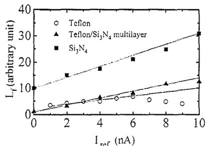
Fig. 6. Friction coefficients of Teflon,  $Si_3N_4$  and  $Si_3N_4$ /Teflon multilayer in nanotribology test.
