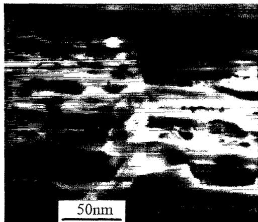
Fig. 2. Fracture surface of TiC/Teflon multilayer with  $t_{\text{TiC}} = 120$  nm and  $t_{\text{Teflon}} = 40$  nm.
