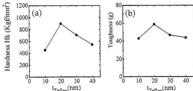
Fig. 3. (a) Hardness and (b) toughness of TiC/Teflon multilayers as a function of the thickness of Teflon layers. (Thickness of TiC layers are constant at 60 nm.)
