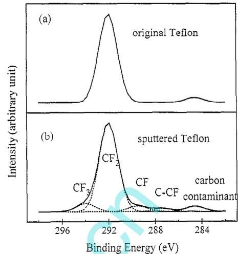
Fig. 1. XPS C1s of (a) original Teflon material and (b) the sputtered Teflon film.
