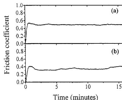
Fig. 5. Friction coefficient of (a) pure TiC and (b) TiC/Teflon multilayer with  $t_{TiC} = 90$  nm and  $t_{Teflon} = 30$  nm.
