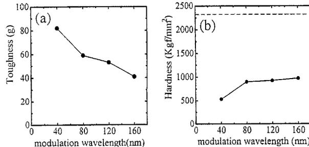
Fig. 4. (a) Hardness and (b) toughness of TiC/Teflon multilayers as a function of the modulation wavelength when the component fraction is the same (75 vol.% TiC).
