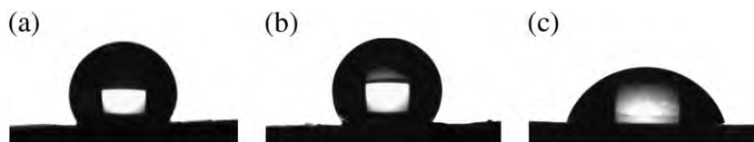
Fig. 6. Water droplet on nickel surfaces with octadecanethiol films with different microtextures. a) Replica of rice leaf. b) Replica of lotus leaf. c) Smooth nickel coating without octadecanethiol film.
