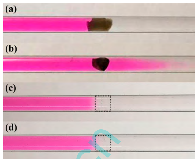
Figure 4. Liquid microvalve fabricated by the MoS 2 /PNIPAM composite hydrogel (a, b) and pure PNIPAM hydrogel (c, d). The photographs show the microvalve before (a, c) and after (b, d) exposure to NIR irradiation (808 nm, 0.8 W) for 2 min. The solutions encapsulated in the left and right sides are a red rhodamine solution and water, respectively.
