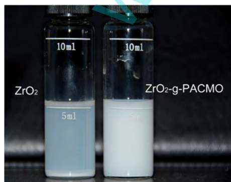
Fig. 4 Sedimentation tests of ZrO_2 and ZrO_2 -g-PACMO nanoparticles in DMF after 24 h.
