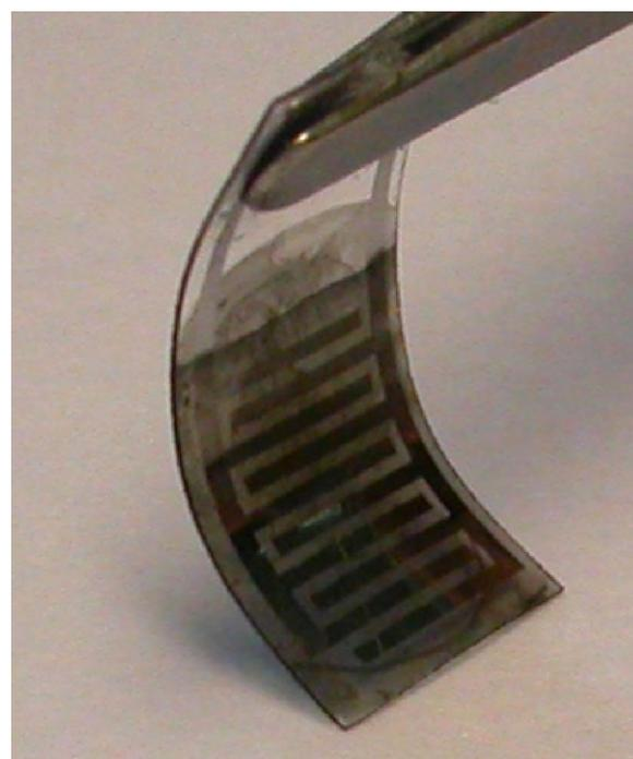
**Fig. 2.** Photograph of bent flexible NH<sub>3</sub> gas sensor based on PPy thin film assembled *in situ* on modified PET substrate.
